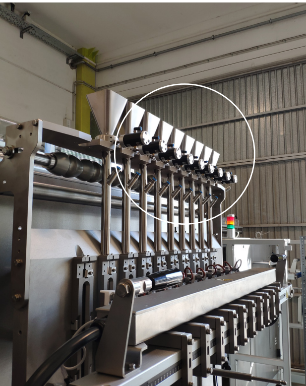
K (linear pneumatic vibrator) - Hopper emptying
