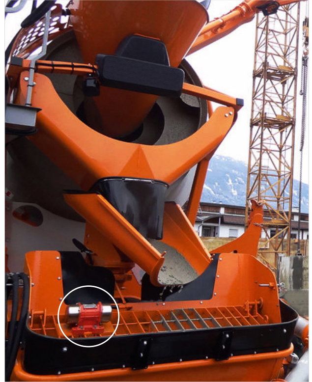
MVE-DC (electric vibrator) - Concrete pump
